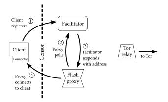
Step 4: The flash proxy connects to the client. The connection is received by a small *connector* program running on the client.
