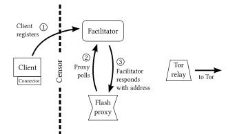
Step 3: The facilitator sends the client's previously registered address.
