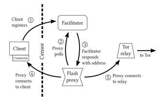
Step 5: The flash proxy makes a second connection to a Tor relay, and begins proxying ciphertext between the client and the relay.
