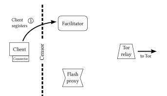
Step 1: A client indicates its need for a connection by registering with a *facilitator*.
