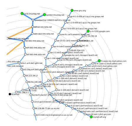
The topology display shows the scanning host, the targets, and all the intermediate hosts that traceroute was able to find. Clicking on any host recenters the graph to radiate outward from the host selected, showing the network from its point of view. Above is a map of the routes to several major web servers from the author's home computer.
