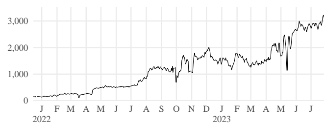
Figure 9: Snowflake users in China. Though no sustained blocking is evident, disruption of domain fronting rendezvous for three days in May 2023 briefly depressed user numbers.
