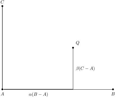
With this setup, it turns out that we can figure out the "coordinates" of Q in the new view rectangle coordinate system quite easily, as follows. We express the vector Q - A as the sum of two vectors, one being a multiple of B - A, and the other being a multiple of C - A, namely let
